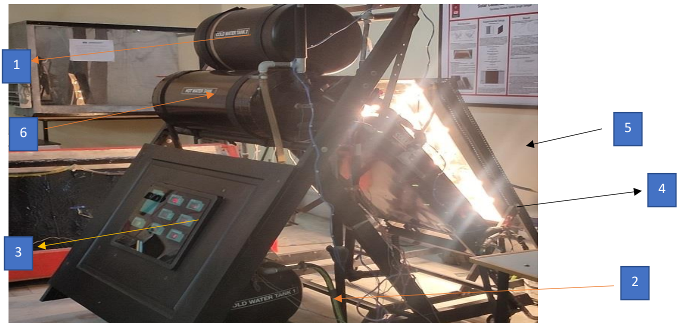
Fig.1 Flat Plate Collector. 1,2. Cold Water Tank 3. Digital Indicator Display 4. Absorber Plate 5. External Radiation Panel 6. Hot Water Storage Tank [3]
