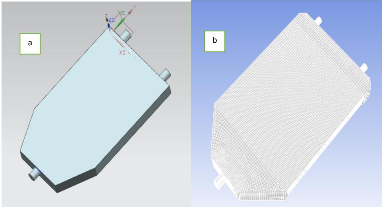
Fig 2. (a) 3-D modelling of a FPC in NX CAD (b) Meshing Grid in Ansys fluent 15.0
