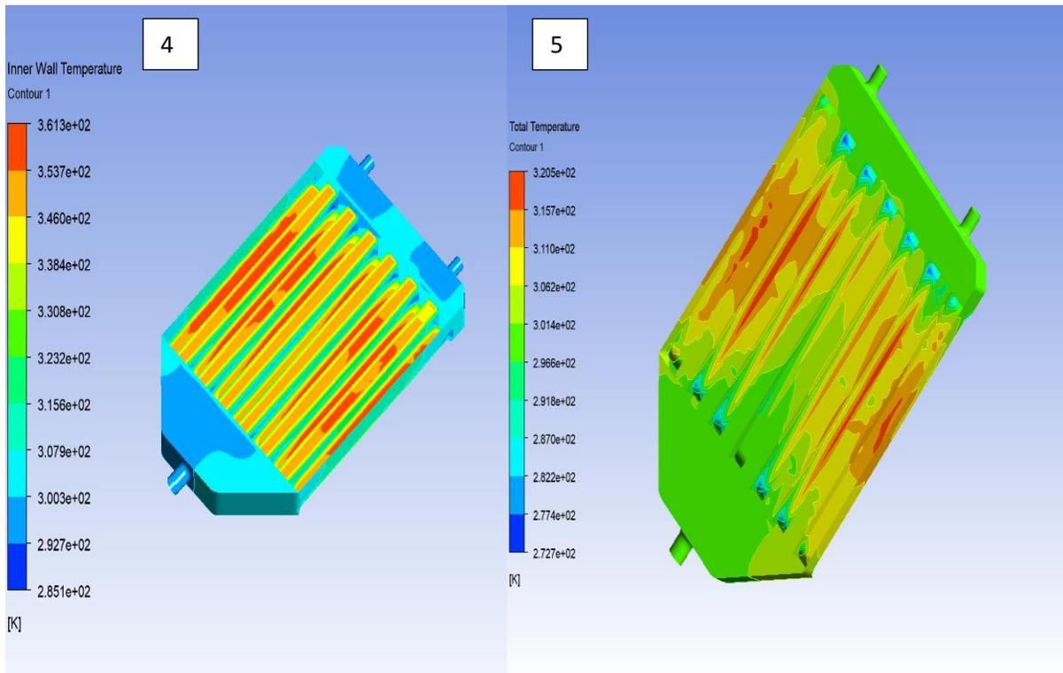
Fig. (4) Variation of Inner Wall Temperature (5) Variation in Total Temperature of FPC
