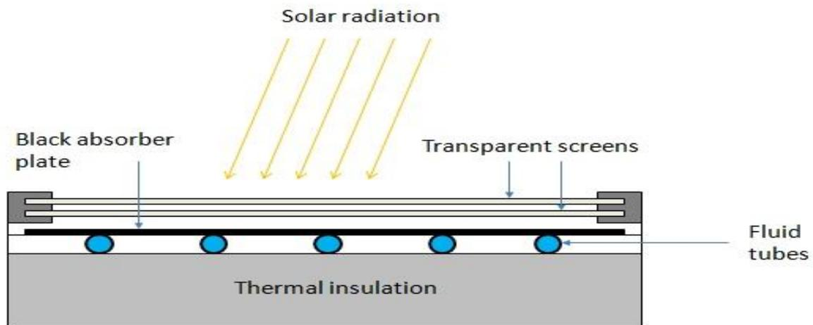
Fig.1 Schematic diagram of double-glazed Flat Plate Collector
