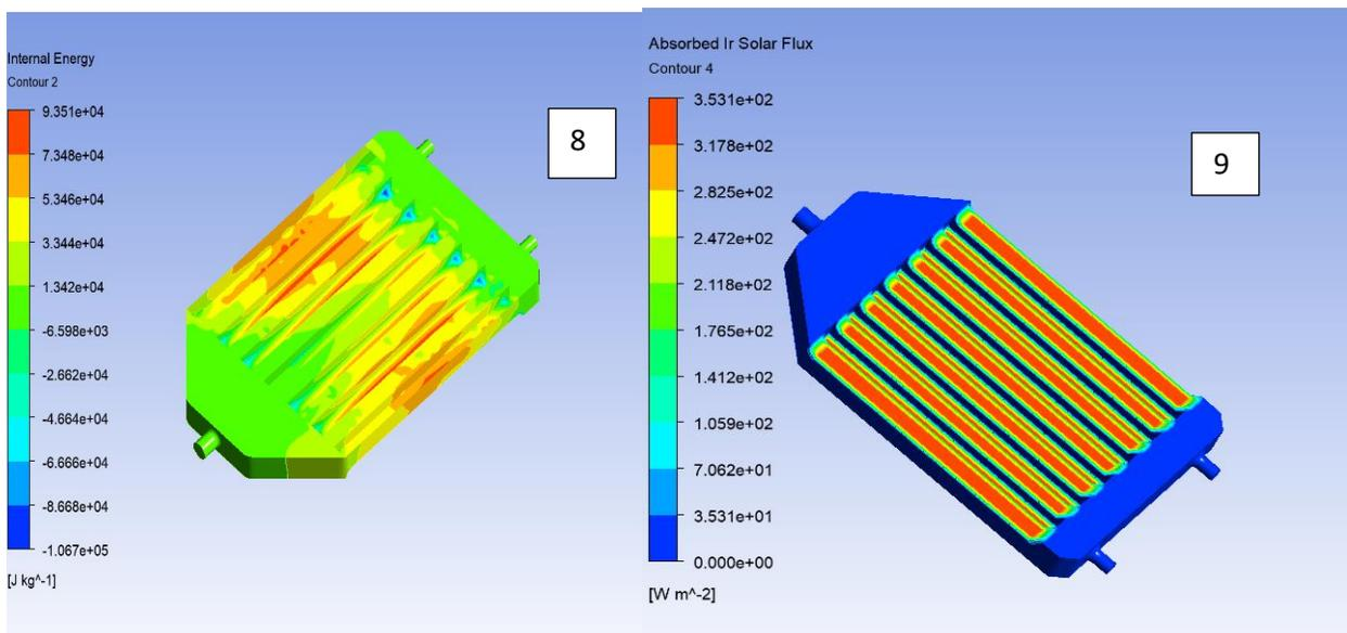
Fig. Variation in (8) Internal energy of FPC (9) Absorbed Solar Flux by FPC
