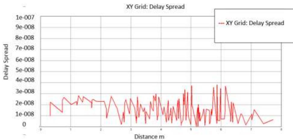
Figure 9. Scenario 2 - Delay spread versus Tx-to-Rx separation distance.
