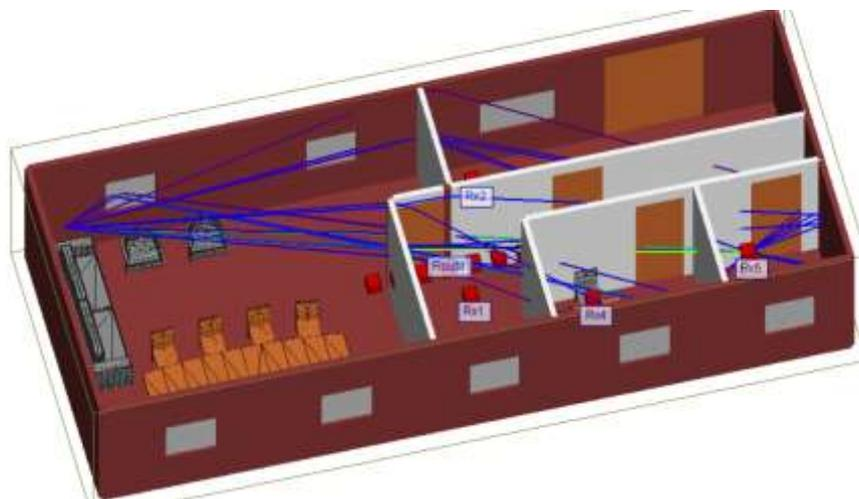
Figure11. Scenario 2 - Illustration of Propagation paths for receiver No.5
