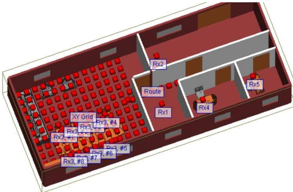
Figure 2. Placement of Transmitter and Receivers Antenna in the office
