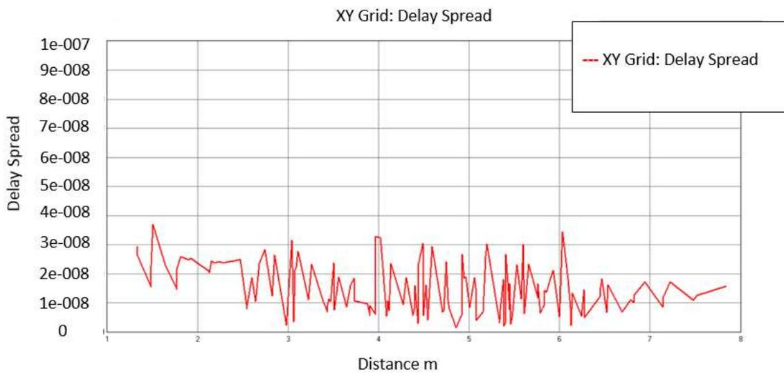
Figure 4. Scenario 1 - Shows the Delay Spread for different Distances of Tx-Rx
