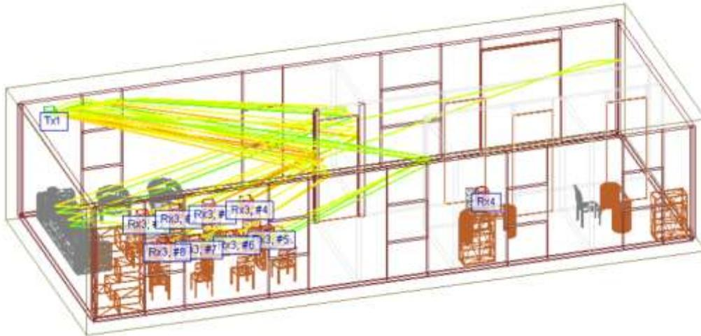
Figure 3. Scenario 1 - Propagation paths from the transmitter (2.9 height) to different received points
