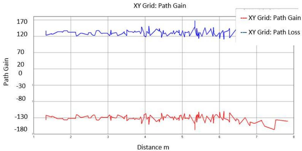
Figure 5(b). Scenario 1: Path loss and Path gain for Scenario 1
