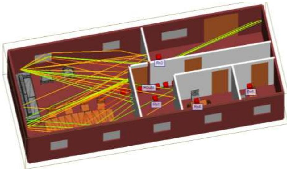
Figure 8. Scenario 2 - Strong propagation paths for transmitter to receivers placed on the table
