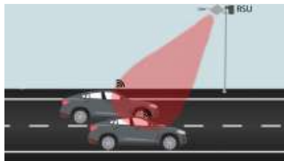
Figure 2. RFID Reader with directional antenna on only one side of the road
