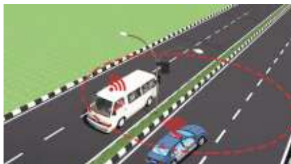
Figure 3. RFID Reader with omnidirectional antenna installed in the middle of the road
