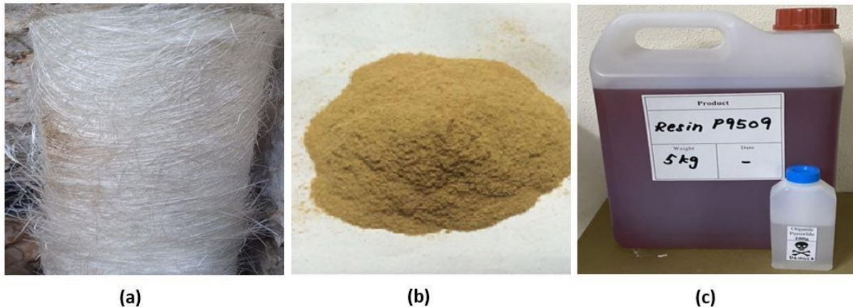
Figure 1. Showing (a) Chopped glass fiber, (b) grounded walnut filler and (c) polyester resin
