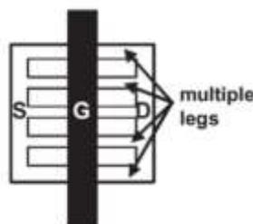
Figure 4. Top view of multiple Tri-gate legs [2]
