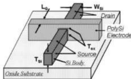
Figure 3. Tri-Gate Transistor Schematic [2]
