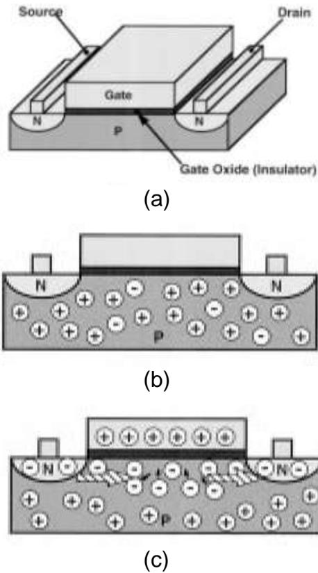
Figure 1. NMOS transistor. (a) Basic Structure. (b)  $V_{gs} = 0$  (c)  $V_{gs} > 0$  [3]
