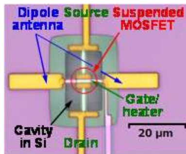
Figure 4. Optical micrograph of the SOI MOSFET bolometer.
