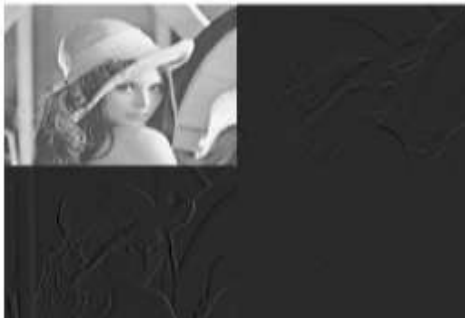
Figure 5(b). 2 Level DWT applied on Water Marked (Lena + Cameraman)
