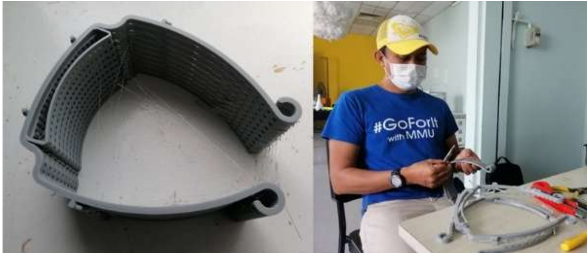
Figure 7 Stack of face shield and the process of removing the support structure.
