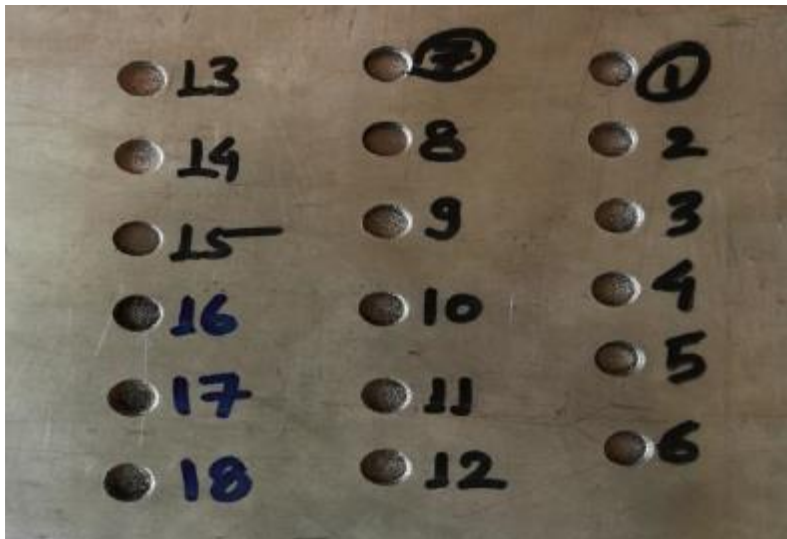
Figure 4: Image of work-piece after L18 experiment in EDM
