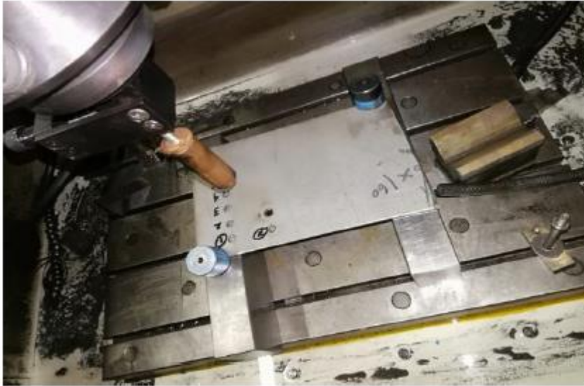
Figure 2: Experimental setup of Copper tool and Workpiece
