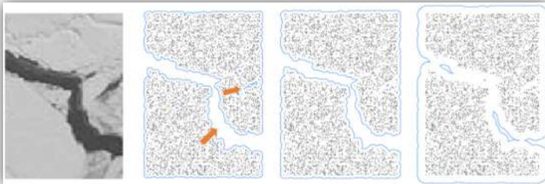
Fig.4. The \alpha -shapes used to discover a way through the ice pack.
