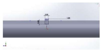
To create crack 2mm here need to create a rectangle shape with dimensions of 2mm, and insert it into beam with 2mm length , after creating it then cut the object with extrusion cut option,
