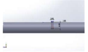
To create crack 6mm here need to create a rectangle shape with dimensions of 2mm, and insert it into beam with 6mm length , after creating it then cut the object with extrusion cut option,
