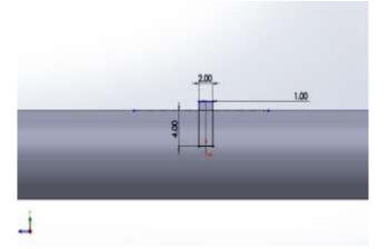
To create crack 4mm here need to create a rectangle shape with dimensions of 2mm, and insert it into beam with 4mm length , after creating it then cut the object with extrusion cut option,
