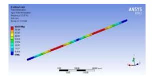
Above image shows the frequency values of beam without crack, and it has material steel 416, at mode3 it has frequency value of 123.87 Hz
