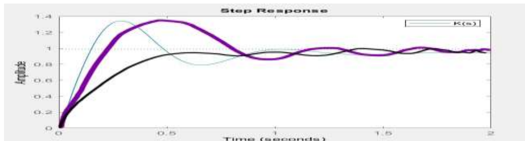
Fig 13. Unity step response of H \infty control for Buck-Boost Converter
