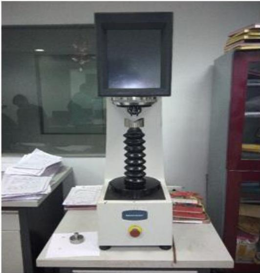
Fig. 3 Brinell hardness tester
