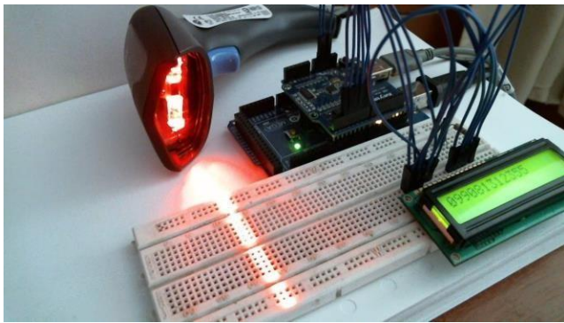
Figure4: Interfacing barcode scanner with Arduino.
