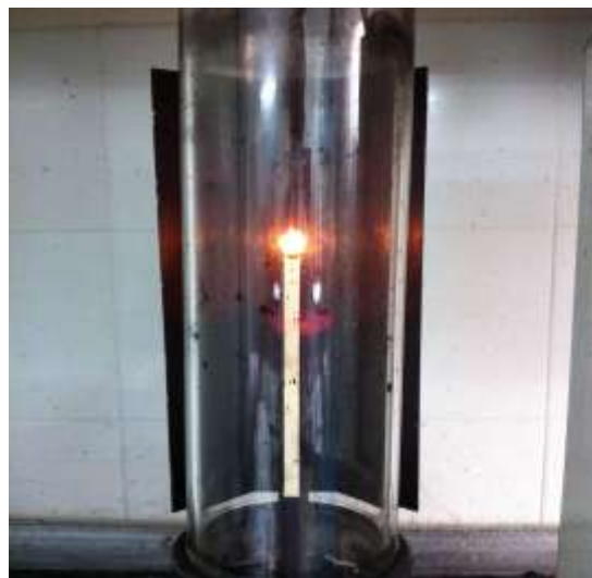
Figure 7. Results for flammability tests (reaction to small flame) oxygen index (OI)
