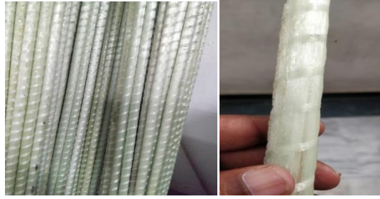
Figure 5: Glass fiber rebar of 12mm diameter
