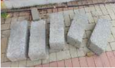
Fig. 5. Curing of the Paercrete.
