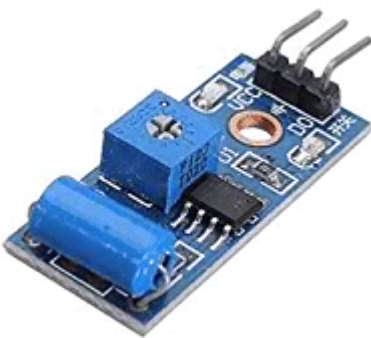
Figure 2:Vibration module based on vibration sensor
