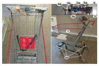
We built a prototype to test our design and functionality. Fig. 3 shows the components of
