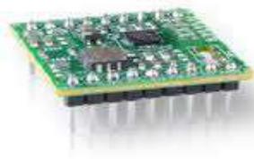
Figure 1. MEMS Sensor which monitors the in-bed posture of the patient.
