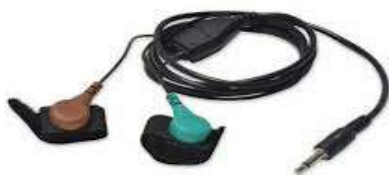
Figure 2. GSR Sensor which records pain level of the patient.
