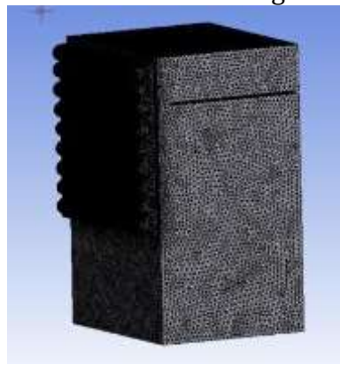
Figure6: Meshing:TotalNo. ofNodes: 366357&TotalNo.Elements:1848509.
