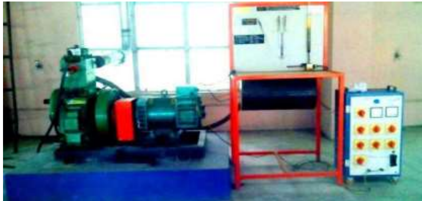
Fig 5 Engine with dynamometer and Gas analyzer
