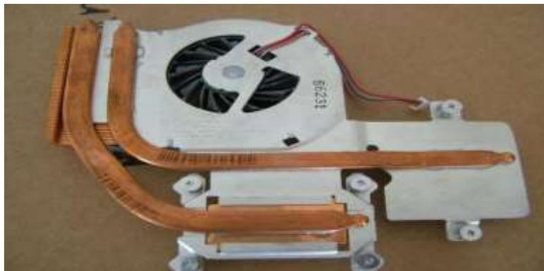
**Figure1.5:** Heat Pipe (Actual photograph)
