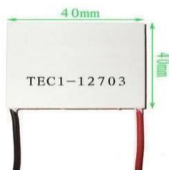
C. Peltier cooler
